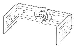
2. Fasten the mounting brackets to the bracket for wall mounting using the fastening screws. The brackets' position can be freely adjusted. We recommend maintaining a distance of 45 to 55 cm between them.
