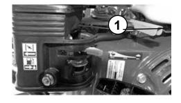
Control drive speed and direction of travel with the handle (1).
