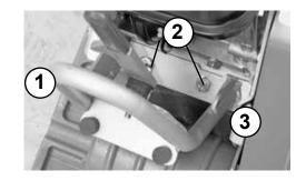
Hook the tank (1) into the holder (2) of the water tank.
