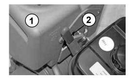
If necessary, cut off the water supply by closing the water valve (1).
