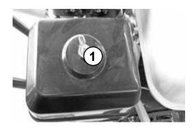
Remove the air filter (1) insert from the air filter enclosure Clean the air filter insert in accordance with theguidelines provided by the engine manufacturer, or replace if there is extreme fouling.
