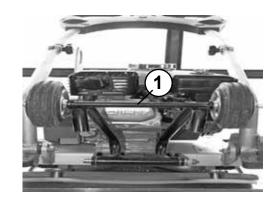
Arrest the hand guidance with the spring bolt(1).
