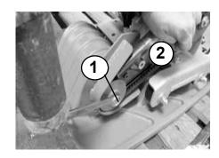
Take off the V-belt pulley (1) and replace the V-belt (1).
