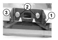
Fasten the chassis (1) inside the chassis mount (2).
