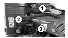
Slowly tighten the handle (1) of the reversing starter (2) until resistance is noticeable.
