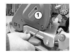
Block the V-belt pulley (1) using a wedge (2).
