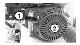
After the engine has warmed up, slide the choke lever to the right (open).
