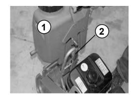
Lock the water tank (1) in place at the tank holder using the lever (2).
