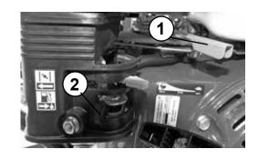
Turn the short-circuit button (1) to the "0" - OFF position.
