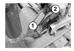
Unscrew the screw (1) on the V-belt pulley (2).
